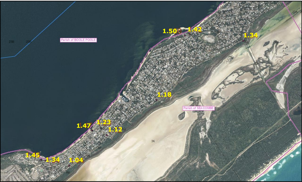
Figure 6: Recorded peak flood levels at Loch Sport, July 2007 flood
